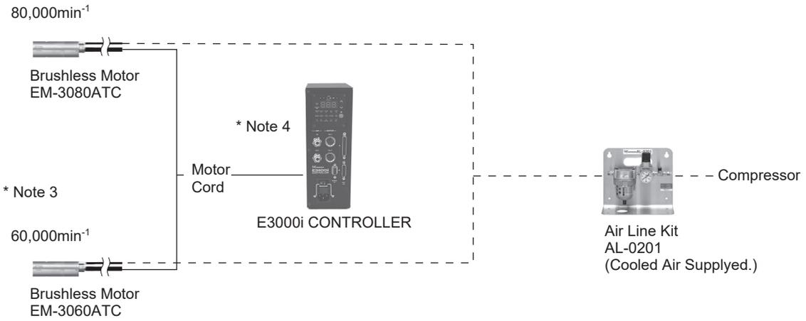
\* Note 3: For the motor for iSpeed5, setting on Parameter  $P_{15}$  is required.
