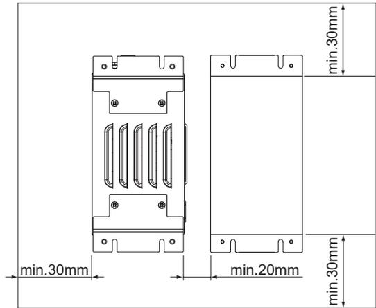
Fig. 25 Horizontal Mounting
