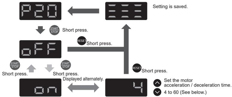
OFF Motor acceleration / deceleration time is set to 2 seconds.
