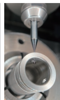
Image of backside deburring in cross-holes
