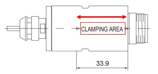
Installing the Grip Ring outside the clamping area may result in premature failure.
