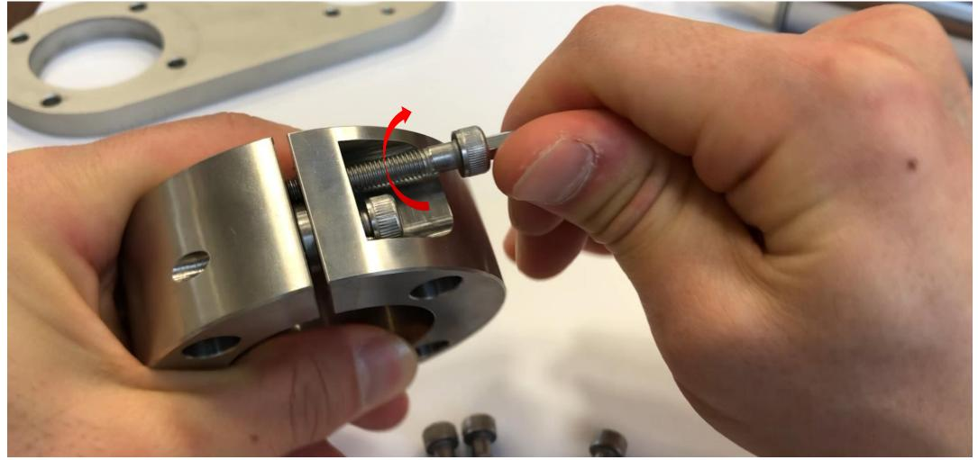
Tighten the provided mounting bolt into the removal screw hole to widen the inside diameter of the Grip Ring.
