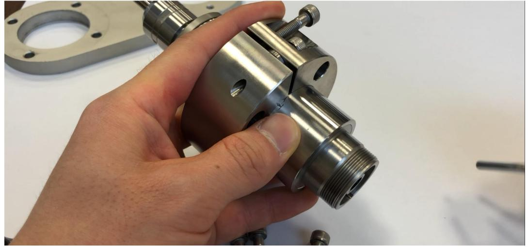
Position the Grip Ring within the clamping area.
