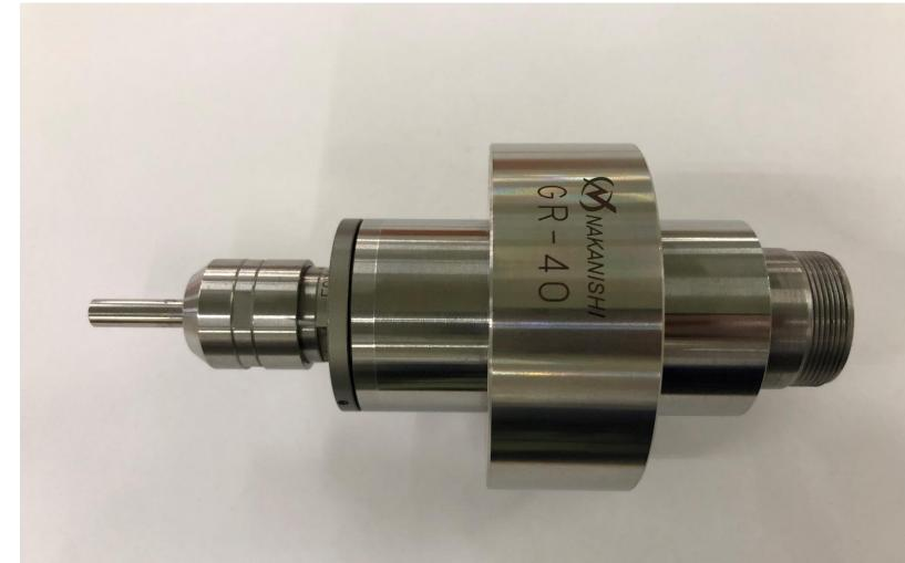
Confirm that the Grip Ring cannot be removed when moved by hand.
