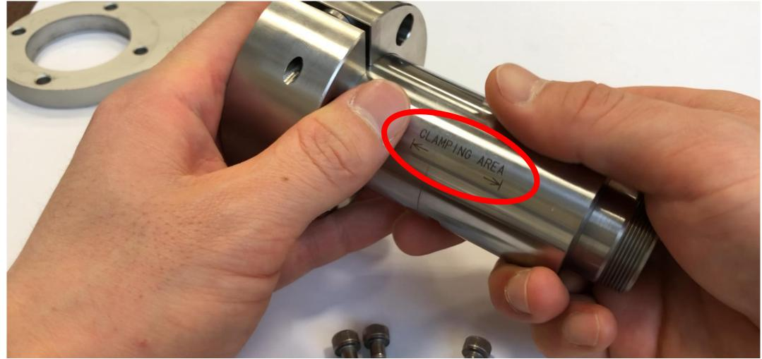
Insert the spindle into the Grip Ring. Confirm the position of the clamping area.
