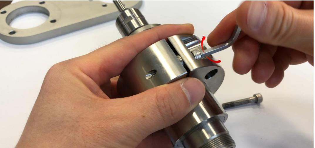
Tighten the lock bolt. The recommended tightening torque for GR-22.8, GR-30, and GR-40 is 4 N·m, while for GR-50 it is 5 N·m.
