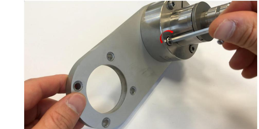
Fix the Grip Ring to the fixing jig with the provided mounting bolts. The recommended tightening torque for GR-22.8, GR-30, and GR-40 is 4 N·m, while for GR-50 it is 5 N·m.
