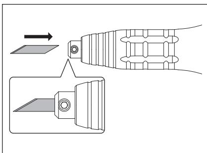
4 Tighten the set screws with a hexagon wrench.
