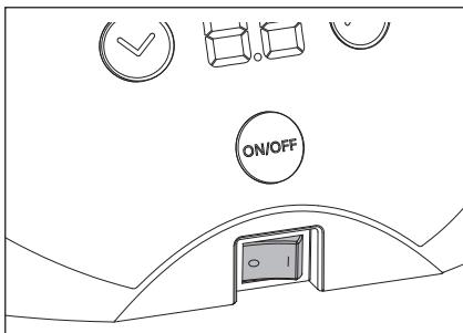
2 While holding down the ON / OFF key (1), turn on the Main power switch (2).
