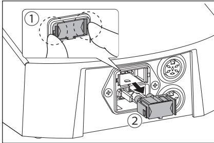
3 Push the claws of the cap firmly into the inlet box.
