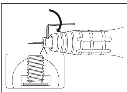
3 If less than 3.0W when the maximum output power is displayed, the blade has been installed correctly. (See "6 - 4 Setting the Watt display and amplitude display.") 3.0W or less is only a guide. It may increase or decrease depending on the surrounding temperature and environment.
