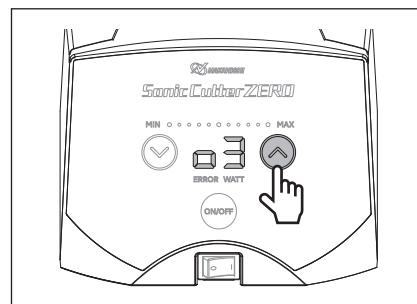
\*1 "o3" is displayed only when it is first set up. After the second time, "o0", "o1", "o2", "o3", "o5", "oR", or "oA", which are stored by the "memory function", will be displayed.
