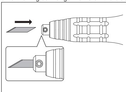
2 Tighten the set screws with a hexagon wrench. When installing a new blade, tighten it in the center so that both ends of the blade do not touch the horn. The standard tightening torque is 1.5 N·m.
