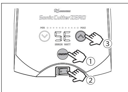
3 Press the UP key to select the item you want to set. The display unit will display the following order\*2: "o3" → "b2" → "P2" → "FO" → "H1" → "o3" → ... Press the DOWN key to change the setting value. When the settings are complete, turn the power off and then on again to complete the settings.
