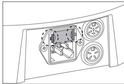
2 Two fuses are used. When replacing them, replace both with the specified fuses.
