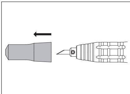
2 Loosen the set screw at the end of the handpiece with the supplied hexagon wrench, and remove the old blade.
