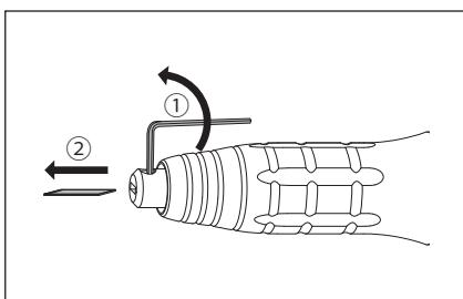
3 Insert the blade all the way into the Horn. The correct orientation is having the set screw clamping onto the Angled Flange Marks on the blade.
