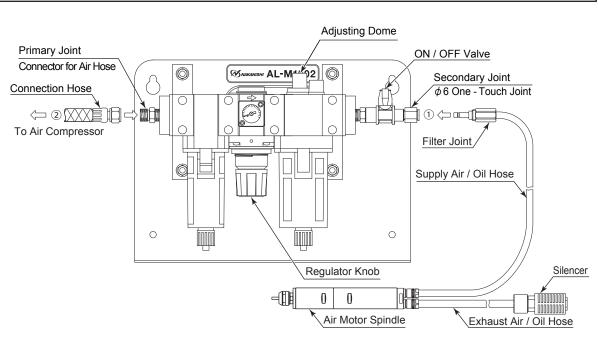
Fig. 20 Connection of Air Line Kit "AL - M1202 (Sold Separately) "
